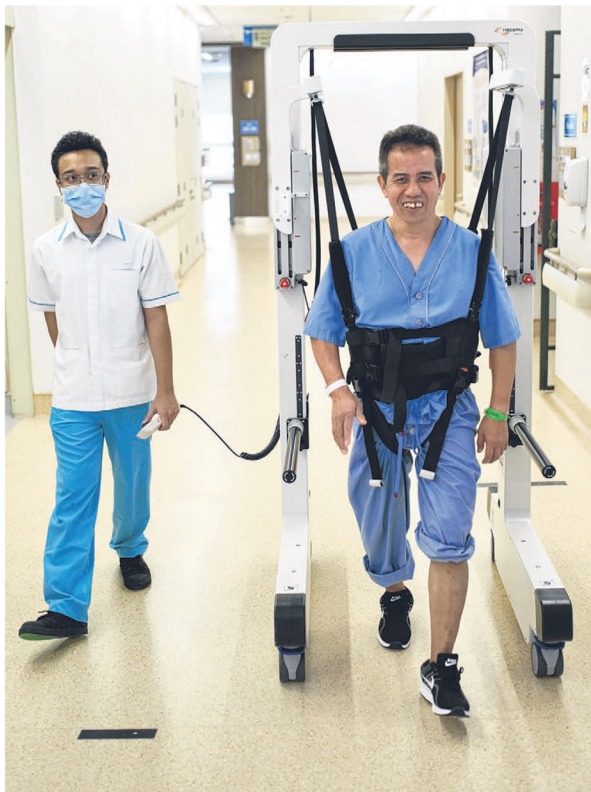
A stroke patient at CGH undergoes rehabilitative therapy using the robotic device, Andago.
